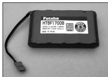
No. F1310 5 Zellen NiMH Akku 1700mAh
